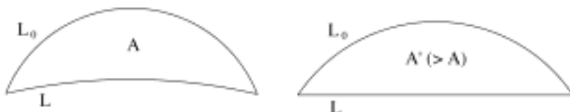
FIGURE 19. Replacing a small portion of a circle on the lid of a cylinder with an arc on the side increases area while maintaining length.
