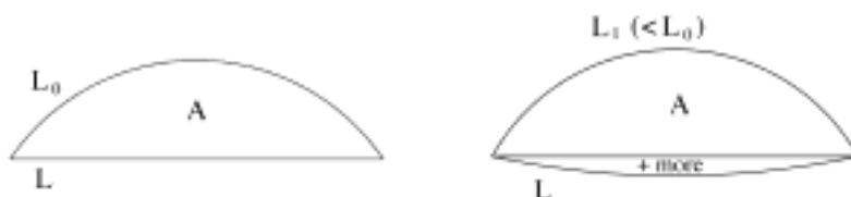
FIGURE 18. Replacing a small portion of a circle on the side of a cylinder with an arc on the lid increases area while decreasing length.
