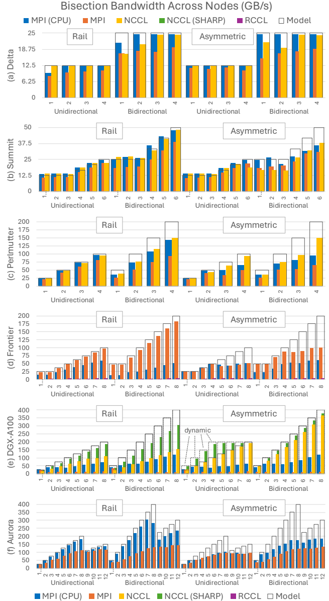
Figure 10. Bisection bandwidth profiles across two nodes were measured with blue (CPU-Only MPI), orange (GPU-Aware MPI), yellow (NCCL), and purple (RCCL) bars. Hollow bars show the proposed model in Equations (1)–(2). Group-to-group patterns gradually change the workload across nodes to expose hardware differences across systems, testing libraries' performance portability and helping developers make choices for moving their applications across systems.
