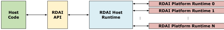
Fig. 16. The three layers in RDAI: RDAI API (interfacing with the host code), host runtime, and platform runtime.
