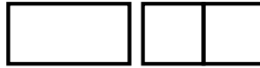
Figure 4.1: Illustration of interval refinement. The high dimensional interval on the left is split into two high dimensional intervals on the right, with respect to the horizontal axis.
