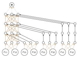
FFNN constructed from RNN with length 4 input sequence, input size of 2, 3 hidden units and output size 1.
