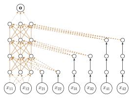
FFNN constructed from RNN with length 4 input sequence, input size of 2, 3 hidden units and output size 1.
