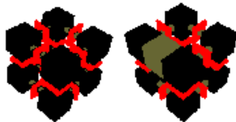
Figure 4: a) Modules and (b) A free block in a 2x2 meta-module configuration.
