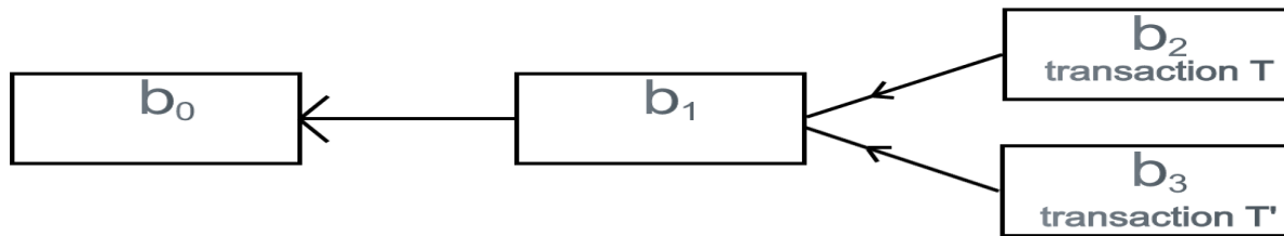
Figure 2: Fork in the blockchain, caused by two new blocks being discovered by different miners at roughly the same time.
