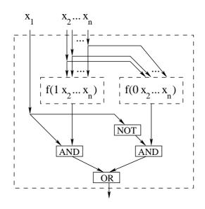
Figure 2: A circuit computing any function  $f(x_1, x_2, ..., x_n)$  assuming circuits for functions  $f(1, x_2, ..., x_n)$  and  $f(0, x_2, ..., x_n)$
