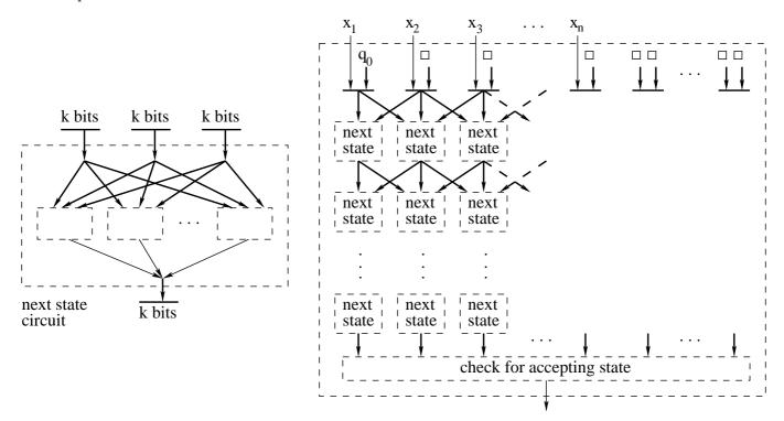
Figure 4: The circuit to simulate a Turing machine M computation by constructing the tableau.
