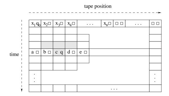
Figure 3:  $t(n) \times t(n)$  tableau of the computation. The left entry of each cell is the tape symbol at that position and time. The right entry is the machine state or a blank symbol  $\Box$ , depending on the position of the machine head.
