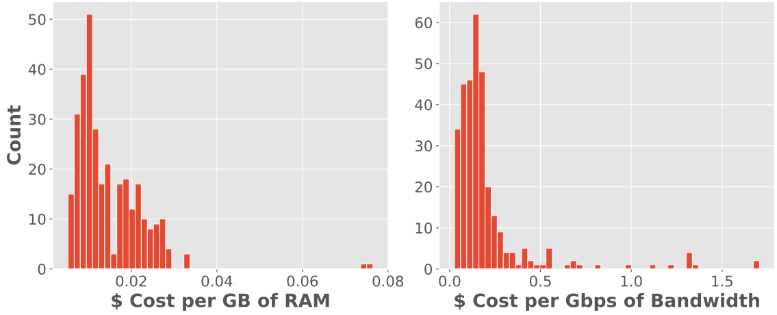
Figure 3.1: Histograms of memory and bandwidth costs of available instance types on AWS.
