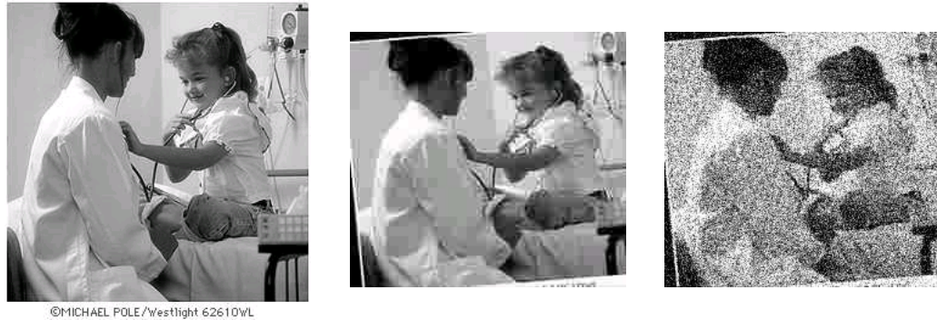
Figure 4.10: Illustration of the canonical attack. From left to right: the original image, the attacked image before adding Gaussian Noise, and the final attacked image
